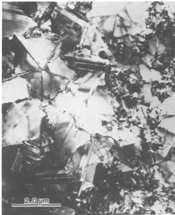
Figure 2 Microstructure of CVD pure nickel.
