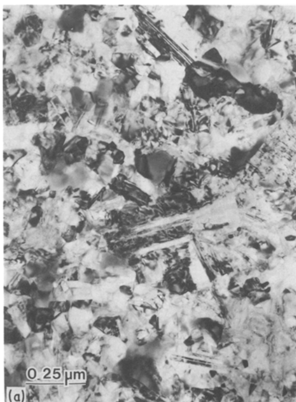
Figure 9 Microstructure of Ni-2.6 at % B after (a) a 1 h anneal at 600°C and (b) following a 600°C, 2.5 h anneal.
